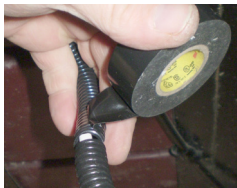
TAPE THE SPLIT LOOM (NOT SUPPLIED)
